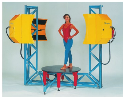
Figure 2. The principle of a laser scanner using a laser as a light source (WB4 from Cyber Ware Company)
